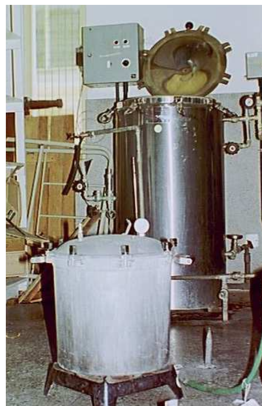
Figure 1 Typical sterilization equipment as used in rural hospitals. The larger sterilizer is a double chamber model. The smaller one is a single chamber model of the pressure cooker type.
